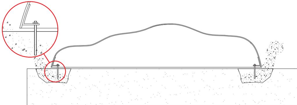
3) A number of threaded rods (corresponding the number of dug holes) is mounted in the internal angles and the StarFish is placed over the holes. The holes are filled with concrete (strength 12).
