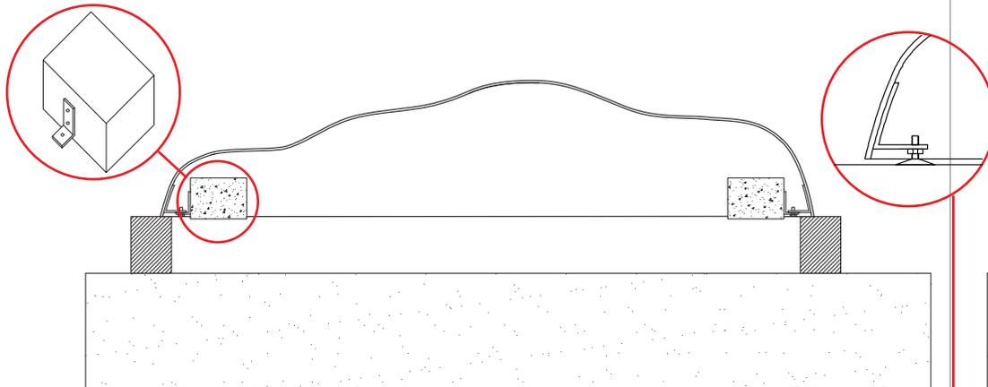
3) Prefabricated concrete blocks are mounted on the 5 internal angles with bolts and nuts. The concrete blocks are wedged up while they are mounted.
