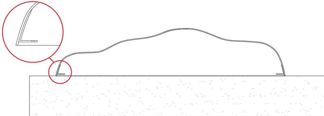
1) StarFish comes with 5 fixed internal angles (stainless steel) with  $\text{\O}14\text{mm}$  holes. Tape markings on the outside of the StarFish indicate the locations of the angles. The tape markings also indicates where to dig holes for the ground foundation.
