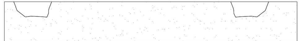
2) Depending on the actual ground conditions dig 5-10 holes for fixating the starfish.
