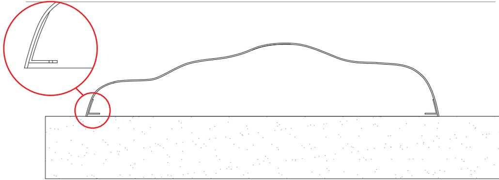
1) StarFish comes with 5 fixed stainless steel angles with  $\text{\O}14\text{mm}$  holes. Tape markings on the outside of the StarFish indicate the locations of the angles.
