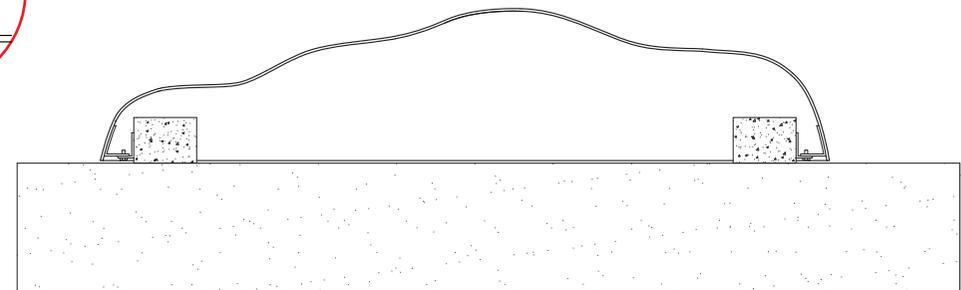
4) The elevation and the wedges for the concrete blocks are removed. The Starfish is fixed and ready for use.
