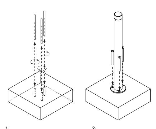
\*Use countersunk bolts (not included) for concrete or equivalent metric bolts with inserts.
