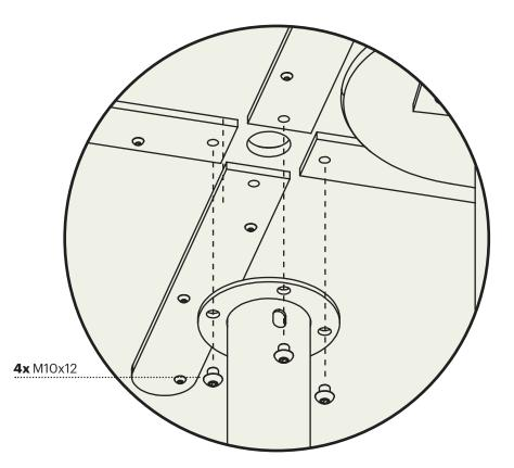
**Fastening of the table** Use M10x12 bolts to fasten the tables to the center tube.
