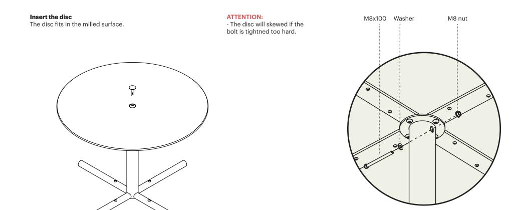
**Fastening of the disc** Use M8x100 bolt, nut and washer to fixate.
