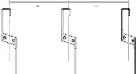
Recommended CC measure between cycling bollards is a minimum of 550 mm.
